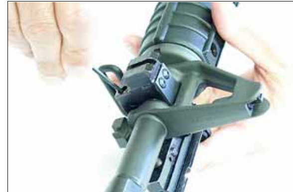
Step 8 - Using the large wrench, run the two shoulder screws through the secondary block into the primary block. Do not tighten. Do Not Use Lock-tite Yet!!!
